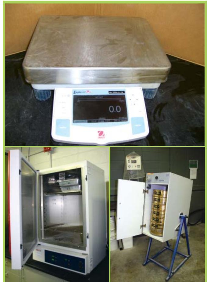
Figure 1. Sieve analysis test equipment
