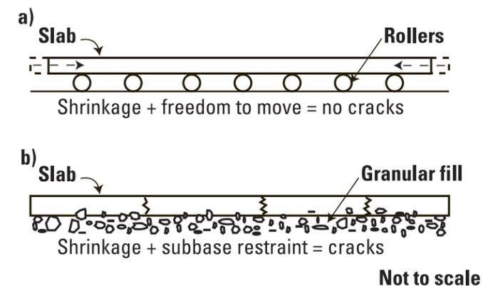
**Figure 1. (a) Cracks generally do not develop in concrete that is free to shrink. (b) In reality, slabs are restrained by the subbase, creating tensile stresses and cracks.**
