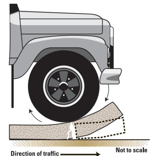
**Figure 2. Curling causes the edge of the slab at a joint or free end to lift off the base, creating a cantilevered section of concrete that can break off under heavy wheel loading.**
