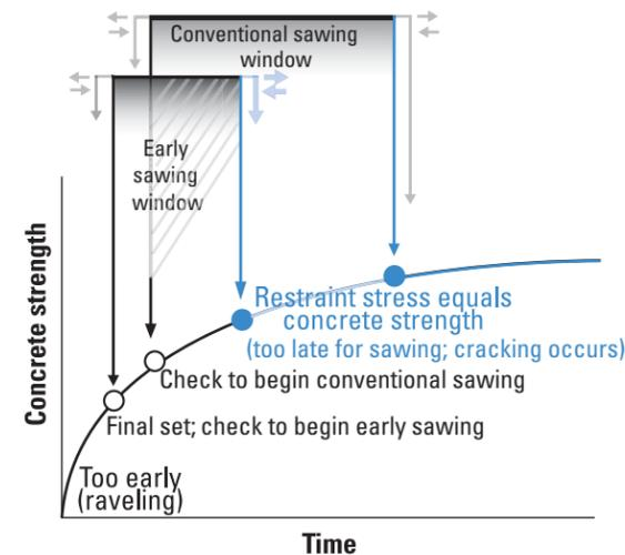
**Figure 3. The exact beginning and end of the sawing window is unique for every concrete pavement system.**
