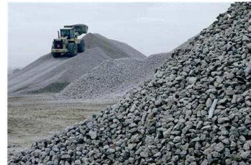
Figure 3. Recycled Crushed Concrete Stockpile
